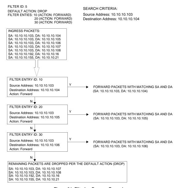
Figure 24: Filtering Process Example
